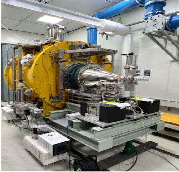
**166 MHz SRF cavity module**
