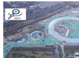
Figure 1. The HEPS building complex. The circumference of the large 1560 m. The extension buildings from this ring will contain three long-bend HEPS, reflecting its magnet design.
