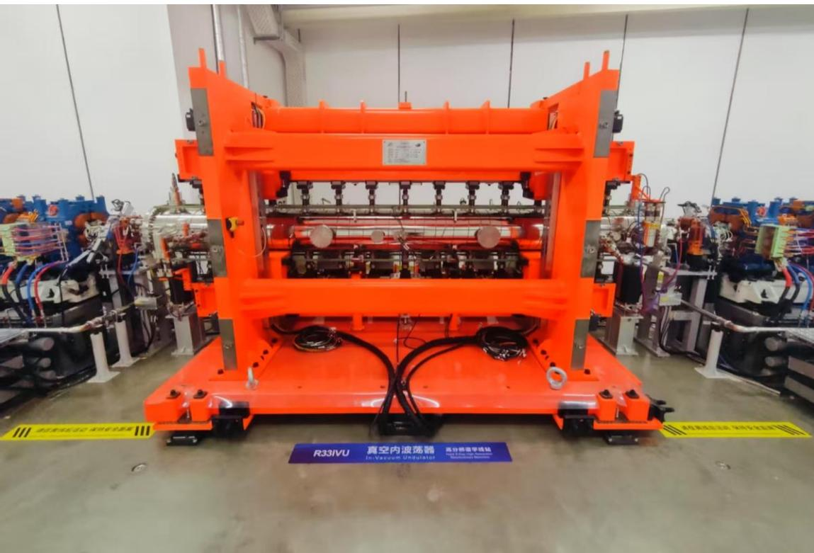
**CPMU** 2m Cryogenic Permanent Magnet Undulator with PrFeB magnet, min gap 5.2mm
