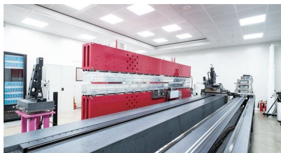
World's first merged four-row APPLE-Knot undulator was under test
