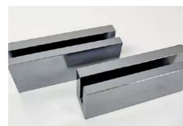
Polishing remotely controlled by magnet field technology was developed to achieve channel-cut crystals with nanometer roughness and strain-free inner surface.
