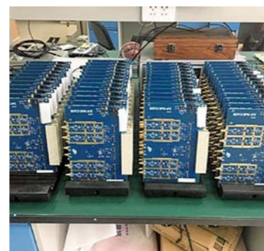
The Beam Position Monitor (BPM) electronics, developed by the Institute of High Energy Physics, operated successfully on BEPCII. The beam position resolution of closed orbit distortion (COD) in the vertical direction was about 21nm by laboratory measurements.
