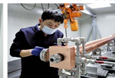
S-band accelerating structures with round-shape cell and internal water cooling had been successfully developed for the first time in China. Matching and cold tests had been completed, and high power test was in progress.
